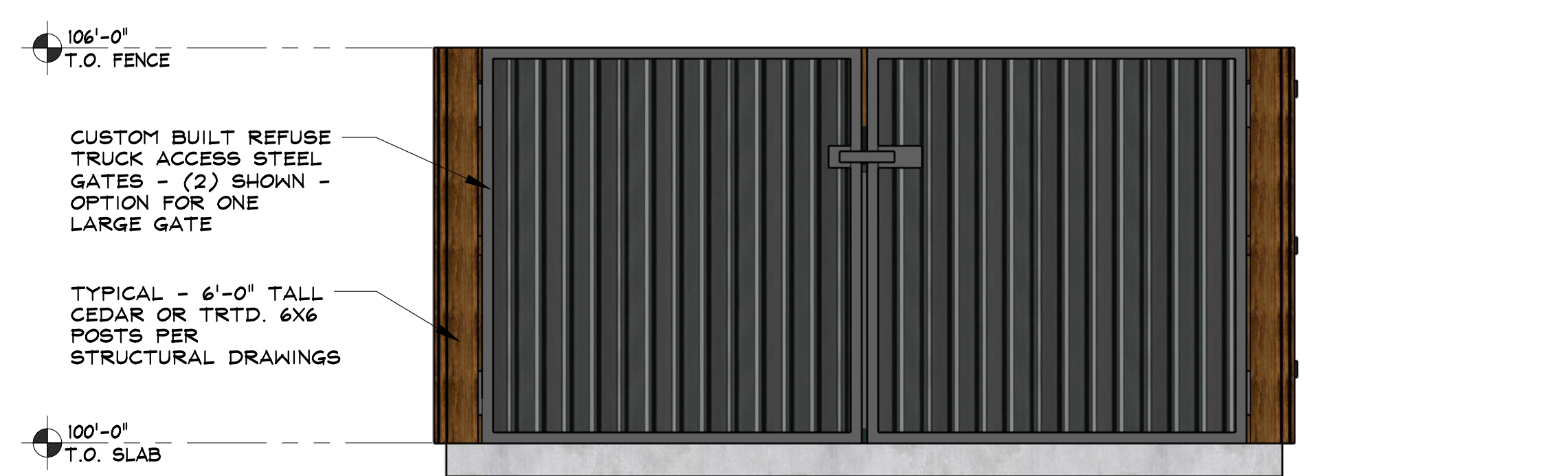
2 CONCEPTUAL FRONT ELEVATION SCALE: 1/2" = 1'-0" NOTES THIS ELEVATION TYPICAL FINAL DOOR SIZES TO BE DETERMINED BY OWNER & CONTRACTOR
