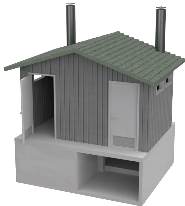
UBC Prescott - 3D Model w/ Concrete Pit
